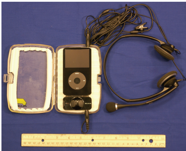
Figure 1. The fly box enclosure with iPod, TuneTalk, and VXi headset/microphone.
