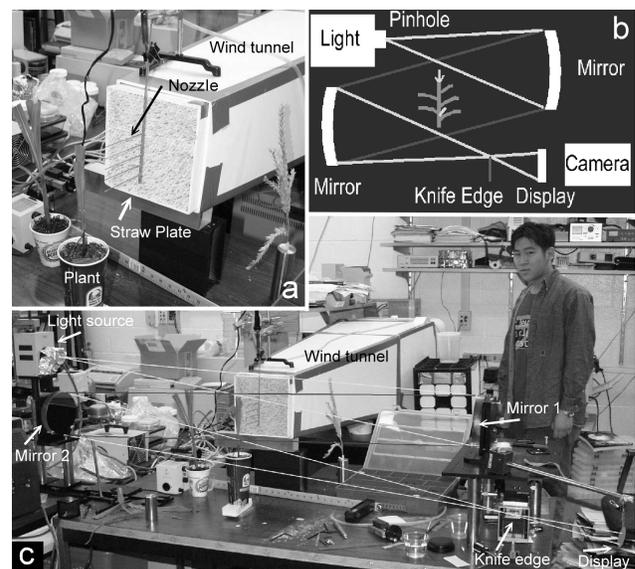
Figure 1. (a) Wind tunnel with straw plate and nozzle. (b) Schlieren optics layout. (c), Schlieren optical setup.
